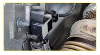
The tubing can be damaged by animal bites or, with advancing age, become porous, leaky and soft, so that it may contract and block the flow completely under slight negative pressure.
