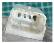
In both cases, it is necessary to clean the tank system and eliminate the cause of the failure. Of course, a professional repair also includes replacing all fuel filters, the fuel pump relay and the crimp connectors that have been damaged by the increased current consumption.
