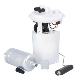
In modern fuel delivery units that still have a return line, leaking fuel tank ventilation hoses in combination with long idle times and low fill levels often lead to severe corrosion in the tank system. This leads to sluggishness of the electric fuel pump and thus to increased power consumption. The resulting heat in turn causes increased resistance, which can be seen at the connector of the delivery unit.
