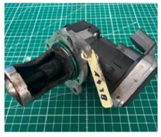
Due to the stricter Euro 6 standard and limited operating conditions, the lowpressure EGR system has meanwhile become standard equipment in every new vehicle. In this system, the exhaust gas is taken only after the particulate filter and, for example, recirculated before the turbocharger. This ensures that the recirculated exhaust gas is cleaned, which prevents coking of the EGR cooler. However, due to the lower exhaust gas pressure in this case, an additional
